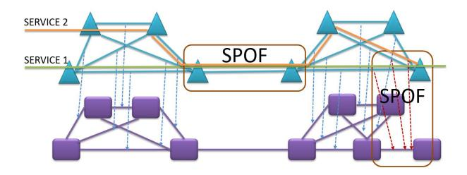
The IMS SPOF functionality performs such assessments. Since IMS understands the protection schemes and the relation between the different networks, IMS will highlight SPOF's after calculating the network topologies and the customer services.
