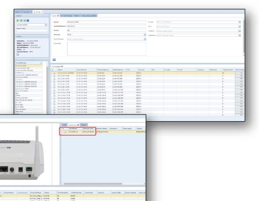
IP addresses can be related to network items, like equipment (loopback address), ports, cards and connections (like VLAN's).
