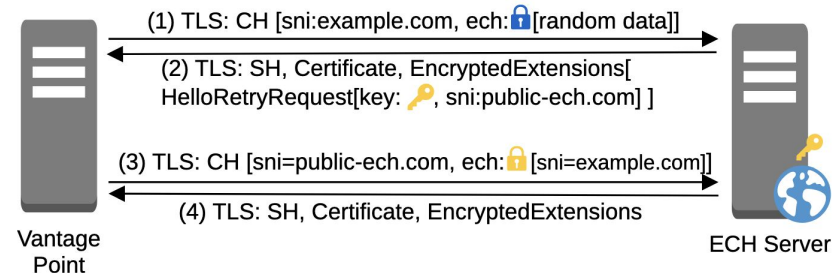
Figure 2: Simplified TLS handshake with ECH in our measurement setup. We use the HelloRetryRequest from the server to determine ECH-capable deployments.
