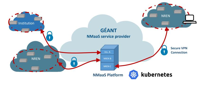
NMaaS uses a secure shared cloud platform managed by the GÉANT Project Each user has a isolated tenant environment connected over a VPN to his network Users can deploy and access network management applications via a web portal
