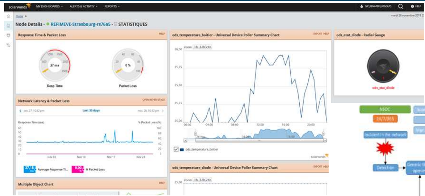
RLS monitoring by the RENATER NOC in Strasbourg (laser diode state at the top right)
