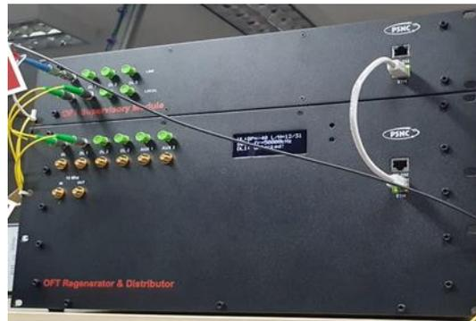
Figure D.3: PikTime Systems Regenerator Laser Station
