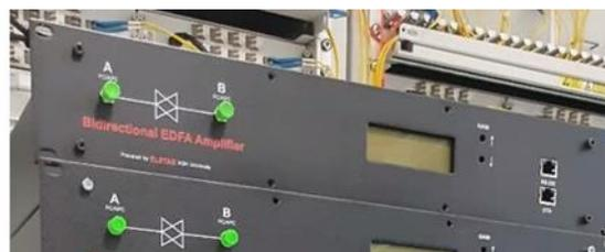
Figure D.2: PikTime Systems bi-directional amplifier
