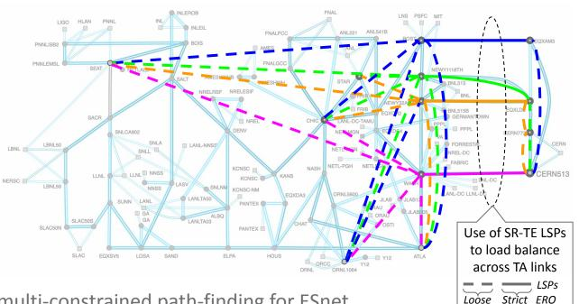
Input as parameter to multi-constrained path-finding for ESnet guaranteed bandwidth dynamic circuit provisioning (i.e., OSCARS).
