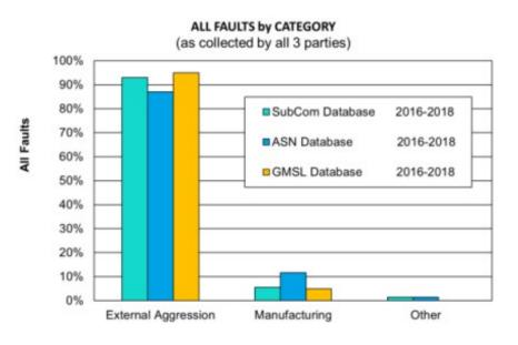
**Overall Causes of Cable Failure**
