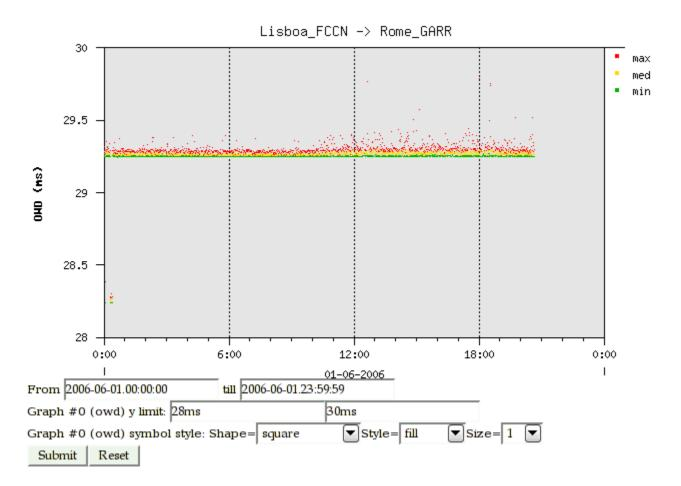
It now becomes evident that most of the samples lie in a very narrow band between 29.25 and 29.5 milliseconds. Interestingly, there are a few outliers towards lower delays. These could be artifacts of clock inaccuracies, or they could point to some kind of routing anomaly, although the latter seems less probable, because routing anomalies normally don't lead to shorter delays.
